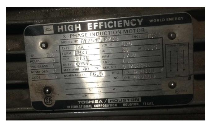
PHOTOGRAPH 6: McPhillips Regional Pumping Station – Air Compressor AC1 Motor Nameplate
